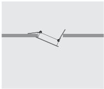
2. Secure the fixture by pushing in the other side.
