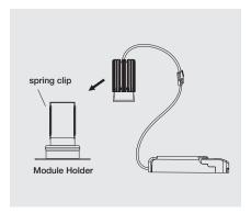
3. Attach module to module holder with spring clip and connect module to driver.
