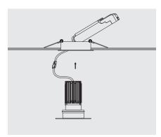
4. Gently insert module holder from the bottom of the fixture frame.
